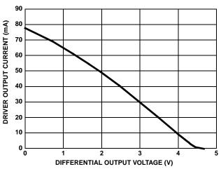
FIGURE 8. DRIVER OUTPUT CURRENT vs DIFFERENTIAL OUTPUT VOLTAGE
