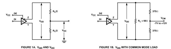
FIGURE 1A.  $V_{OD}$  AND  $V_{OC}$
