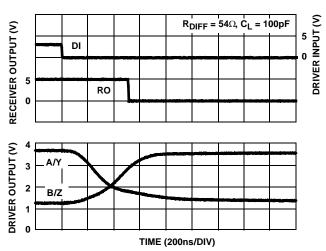
FIGURE 21. DRIVER AND RECEIVER WAVEFORMS, HIGH TO LOW (ISL83083E, ISL83085E)
