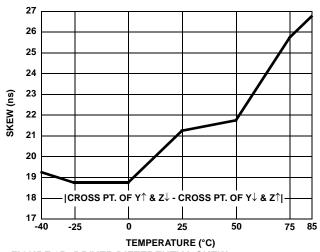
FIGURE 15. DRIVER DIFFERENTIAL SKEW vs TEMPERATURE (ISL83083E, ISL83085E)
