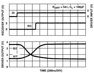
FIGURE 20. DRIVER AND RECEIVER WAVEFORMS, LOW TO HIGH (ISL83083E, ISL83085E)
