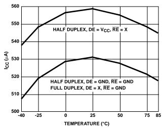
FIGURE 11. SUPPLY CURRENT vs TEMPERATURE
