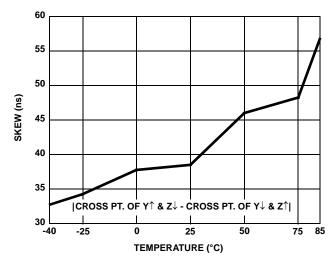
FIGURE 13. DRIVER DIFFERENTIAL SKEW vs TEMPERATURE (ISL83080E, ISL83082E)
