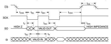
21.3 Waveform 3 – RapidS Mode 0 (F<sub>MAX</sub> = 66 MHz)
